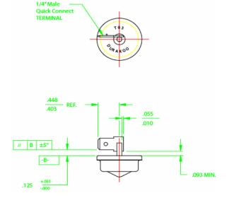
Shown in normally closed position. Tip over switches "break" when the electrode is tilted from the vertical and "make" when returned to the vertical.
